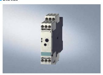
The 3RS10/3RS11 analog temperature monitoring relays can be used for measuring temperatures in solid, liquid and gas media. The temperature is sensed by the sensors in the medium, evaluated by the device and monitored for overshoot or undershoot. When the threshold values are reached, the output relay switches on or off depending on the parameterization.
