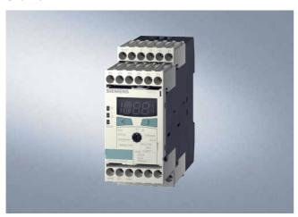
The 3RS10/3RS11 temperature monitoring relays can be used for measuring temperatures in solid, liquid and gas media. The temperature is sensed by the sensor in the medium, evaluated by the device and monitored for overshoot or undershoot or for staying within an operating range (window function).
