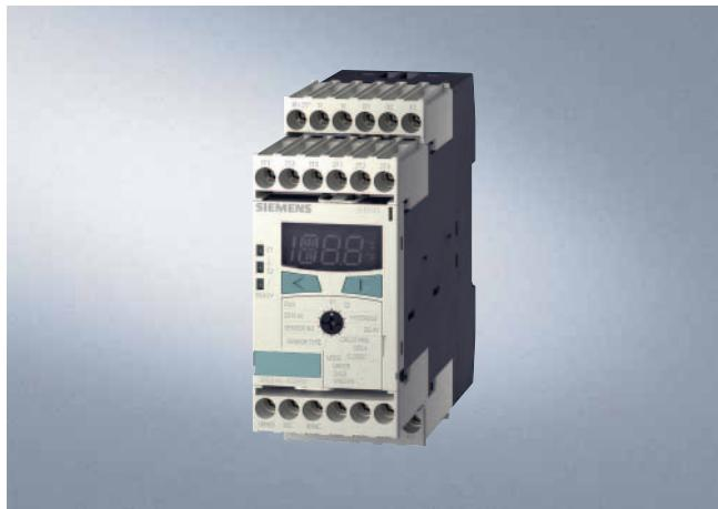
The 3RS10/3RS11 temperature monitoring relays can be used for measuring temperatures in solid, liquid and gas media. The temperature is sensed by the sensor in the medium, evaluated by the device and monitored for overshoot or undershoot or for staying within an operating range (window function).
