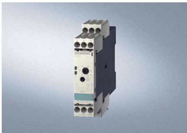
The 3RS10/3RS11 analog temperature monitoring relays can be used for measuring temperatures in solid, liquid and gas media. The temperature is sensed by the sensors in the medium, evaluated by the device and monitored for overshoot or undershoot. When the threshold values are reached, the output relay switches on or off depending on the parameterization.
