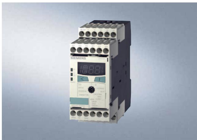
The 3RS10 41 temperature monitoring relays can be used for measuring temperatures in solid, liquid and gas media. The temperature is sensed by the sensor in the medium, evaluated by the device and monitored for overshoot or undershoot or for staying within an operating range (window function). The evaluation unit can evaluate up to 3 resistance sensors at the same time and is specially designed for monitoring motor windings and bearings.
